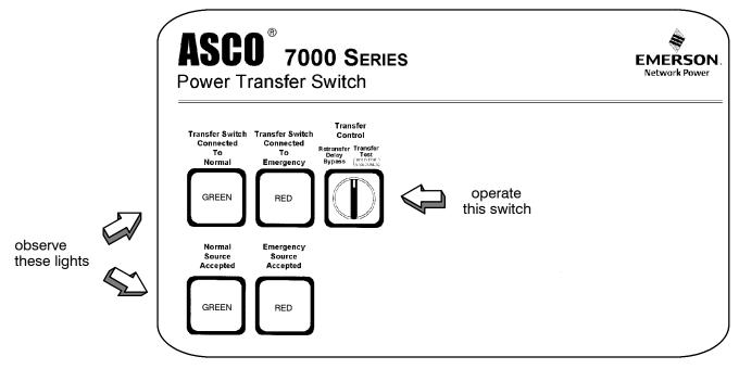
Figure 1-5. Standard controls and indicators.
